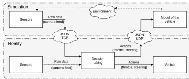
Figure 5: Architecture of the extended HIL scheme [12]
