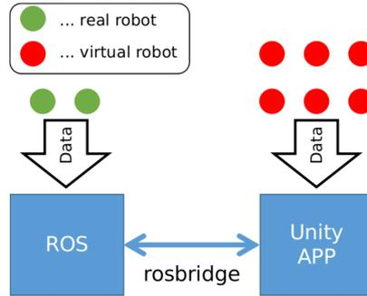
Figure 4: Communication scheme of the multi robot mixed reality test system [9]
