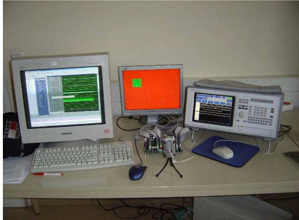
**Figure 1: A Digital Design workplace with development system, target system with attached VGA monitor, and logic analyzer**
