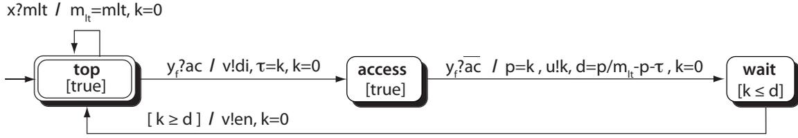
Fig. 7. Automaton for secondary controller  $Q$ .
