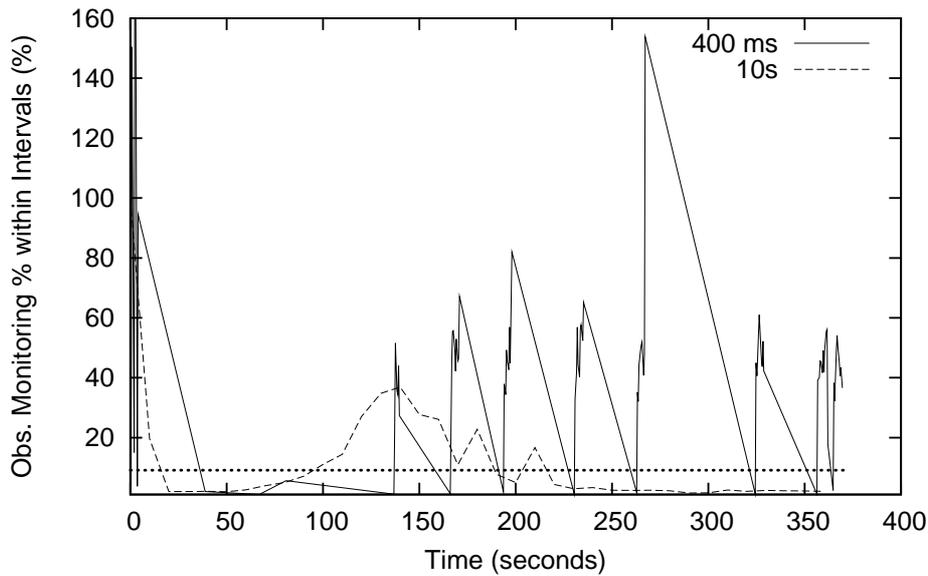
**Fig. 24.** Observed monitoring percentage over `bzip2 range-solver` execution. The percent of each adjustment interval spent monitoring for 2 values of  $T$ . The target monitoring percentage is shown as a dotted horizontal line.
