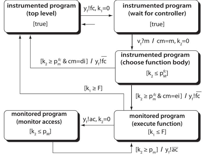
Fig. 4. Automaton for the software plant  $P$  of all monitored objects.
