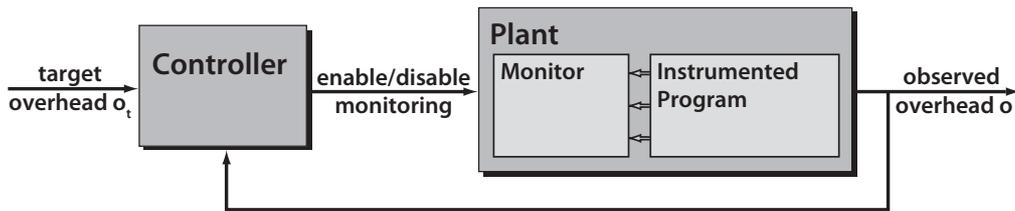
Fig. 1. Structure of a typical SMCO application.
