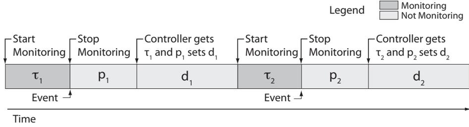
Fig. 8. Timeline for secondary controller.
