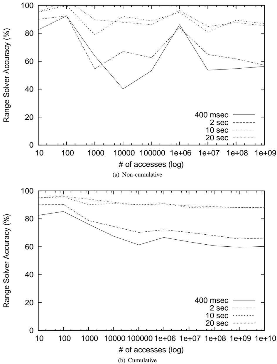
**Fig. 25.** Accuracy of cascade controller  $T$  values with 4 values of  $T$  on the `bzip2` workload using `range-solver` instrumentation. Variables are grouped by total number of updates.
