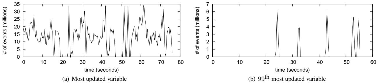
**Fig. 14.** Event distribution histogram for the most updated variable (a) and 99<sup>th</sup> most updated variable (b) in `bzip2`. Execution time ( $x$ -axis) is split into 0.4 second buckets. The  $y$ -axis shows the number of events in each time bucket.
