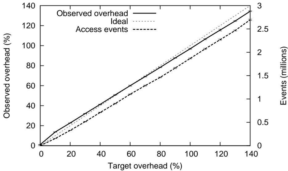
**Fig. 18.** Cascade controller with NAP detector observed overhead ( $y$ -axis) and number of monitored memory access events ( $y_2$ -axis) for a range of target overhead settings ( $x$ -axis) running on the `gzip2` workload.
