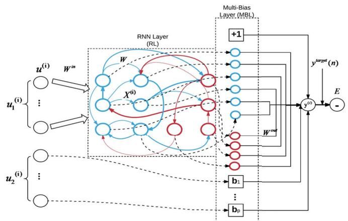
Fig. 1. Multi-Bias Randomly Connected Recurrent Neural Network Structure. Blue neurons stand for excited neurons. Red ones represent inhibited neurons. Bold connections means neurons have stronger impact on others. Thick ones mean less weights values. This figure is only for demonstrating how MBRC-RNN works, it is unnecessary that one places all inhibitory neurons in the right part as depicted in this figure.
