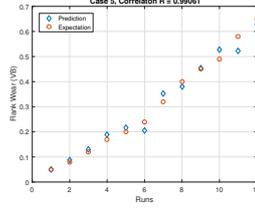
Fig. 8. Case 5 experiment results. The correlation efficient between prediction and desired outputs is  $R = 0.99061$ .
