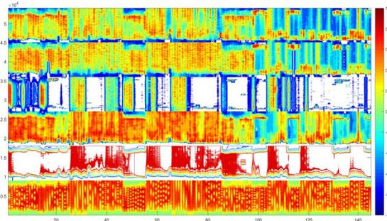
Fig. 2. Contour of normalized experimental data set. Horizontal axis is the index of various runs, vertical axis constituted by spindle motor current, spindle motor current, table vibration, spindle vibration, acoustic emission from table and spindle, respectively.
