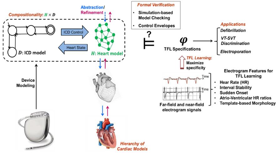
Figure 1: Verification Framework for ICDs
